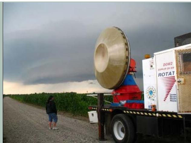
SOARS Student Theresa Aguilar stands by the Doppler on Wheels II as she watches a gust front roll in during the Convective and Orographically induced Precipitation Study (COPS) near the Black Forest in Germany, Summer, 2007.
