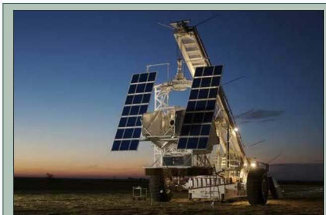
A team of scientists and engineers in EOL and HAO built this 23-foot gondola (seen here with solar panels attached) as part of the Sunrise project, an international program to measure magnetic fields, dynamics, and thermal properties of the solar atmosphere. Carried approximately 25 miles (40 kilometers) into the atmosphere by a giant balloon, the gondola will contain a 1-meter diameter solar telescope that can capture high-resolution images of the Sun's outer surface.
