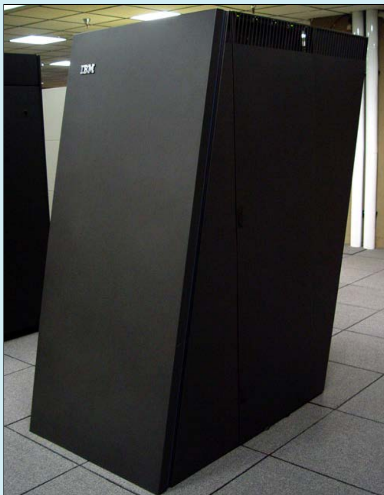
The IBM Blue Gene/L computer "frost" at NCAR was innovative in more ways than just the shape of its cabinet when it was installed in 2005. Its high-performance, low-power-consumption design had great potential, but the system required R&D to become a useful tool for geosciences research. That work has been very successful, and frost is now performing at a high level in multiple roles for universities, NCAR, and the TeraGrid.
