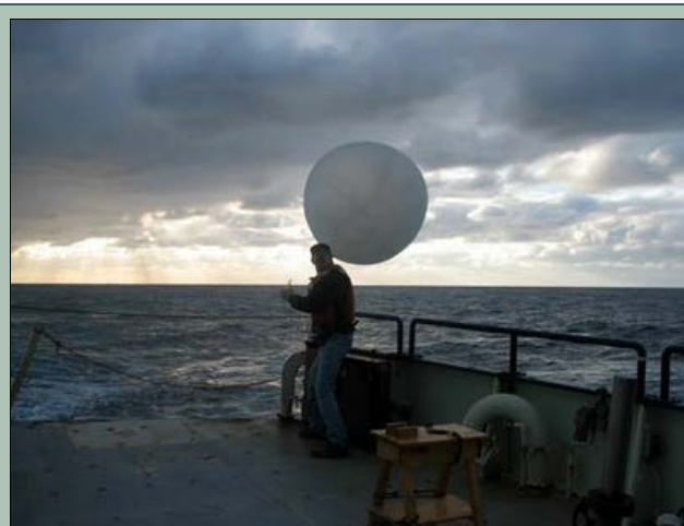
EOL scientist Bill Brown does a last minute check of atmospheric conditions before he launches a sounding balloon off the R/V Knorr during CLIMODE, an experiment which studied the loss of heat from the North Atlantic sea into the atmosphere.
